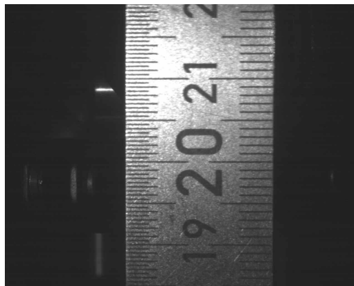
Figure 2.9.: A screenshot of a ruler, taken with the digital camera. The focus of the digital camera is the same as for the screenshots of the MOT. With this image, we can find the correspondence between length and pixels.
