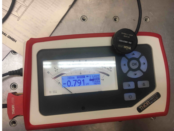
Figure 2.3.: The optical power meter used in this experiment, consisting of the sensor and a display.
