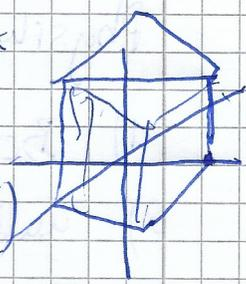
$J_z = \frac{1}{12} \underbrace{ab}_{\substack{\uparrow \\ \text{ab}}} c \rho (b^2 + a^2) = \frac{1}{12} M (a^2 + b^2) \checkmark$
