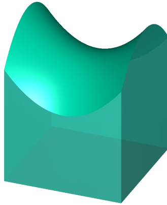
Figure 2.2: Some function z = f(x, y) in a three-dimensional plot. The integral I_2 then yields the volume under the function f(x, y) . For f(x, y) = 1 , one dimension is just the constant function, thus turning the volume into an area in some sense, because V = A \times 1 (1 in the z -direction). Image taken from [7].
